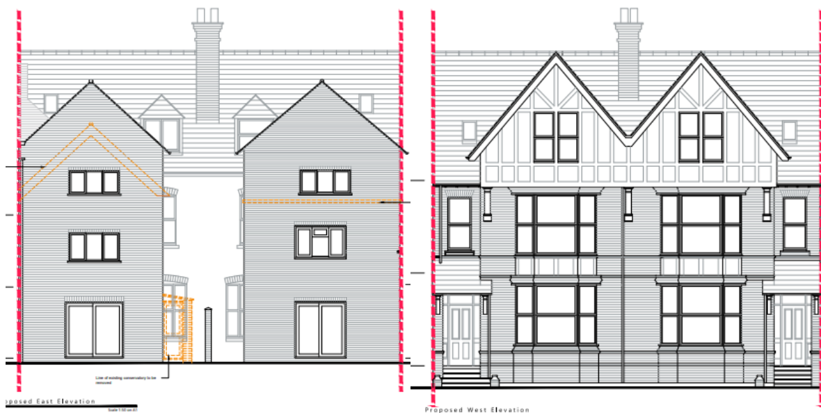
Image 4: Proposed rear and front building façades
