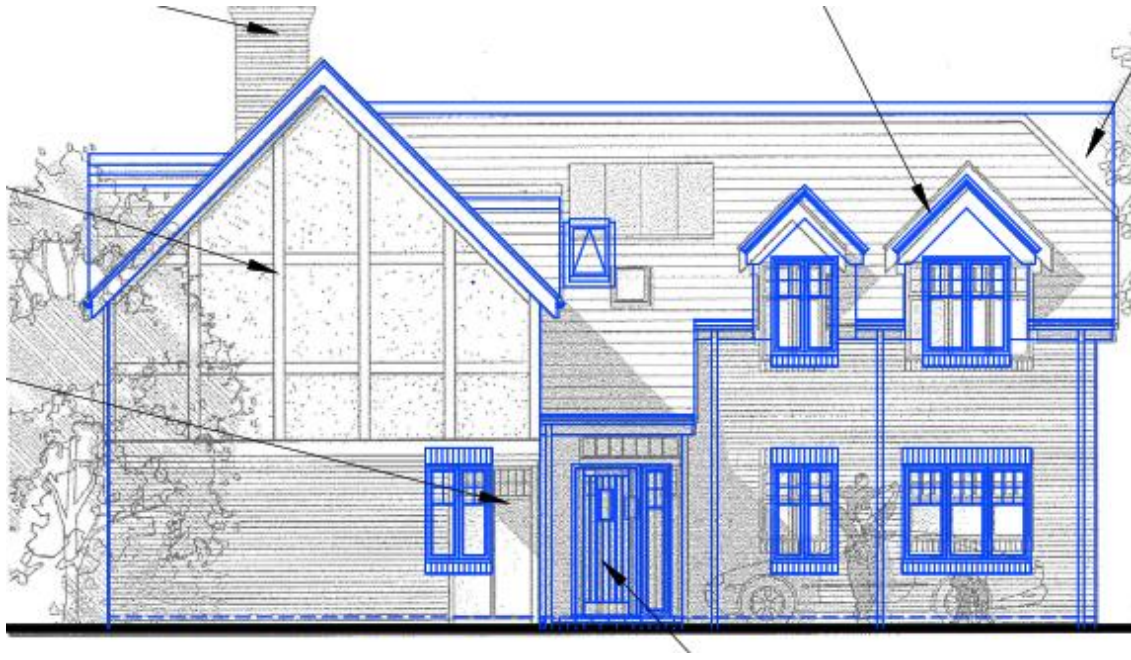
Figure 2 - Proposed south / front elevation (in blue) overlaid over extant permission Note: Elevation facing Woodlands
