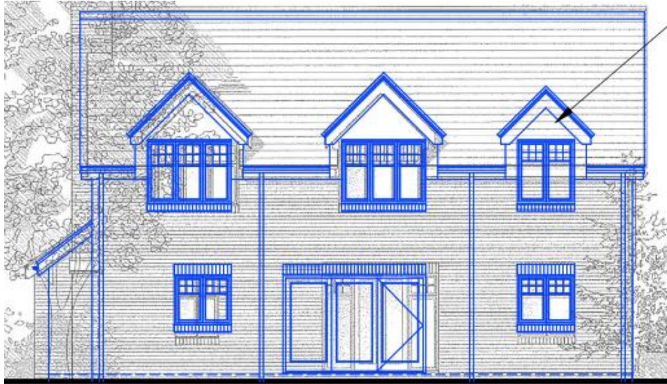
Figure 4 - Proposed west side elevation (in blue) overlaid over extant permission Note: Elevation facing 22 Hudson Close
