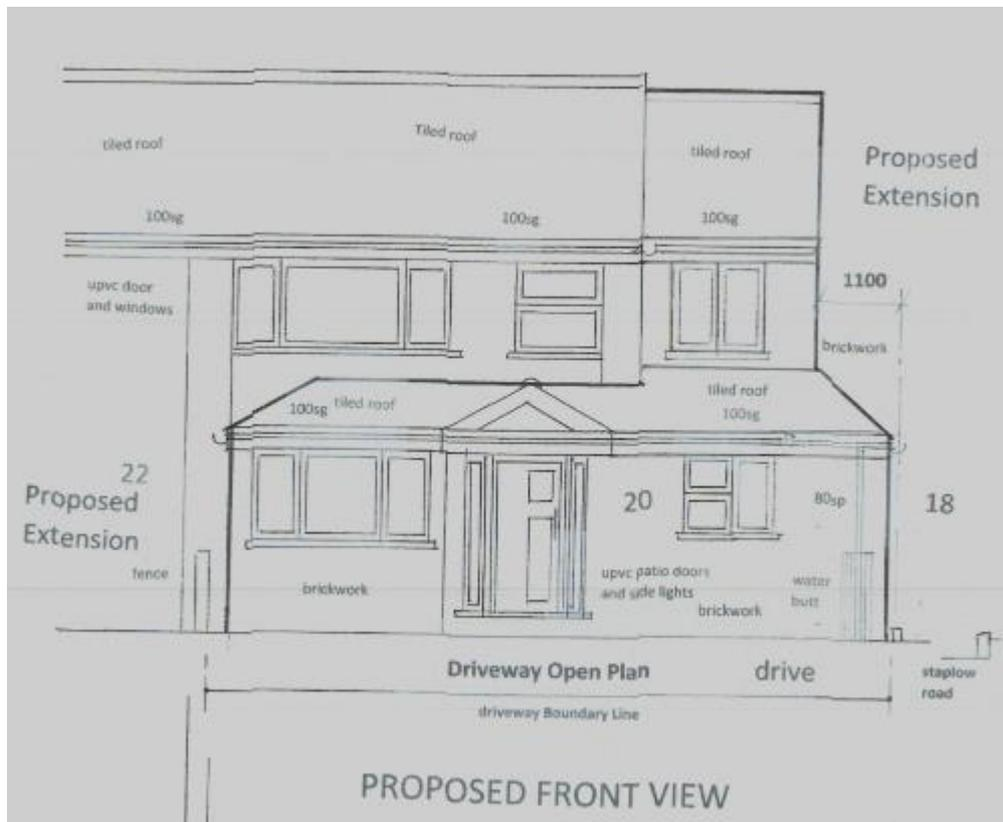
**Figure 2 – Proposed Front Elevation**
