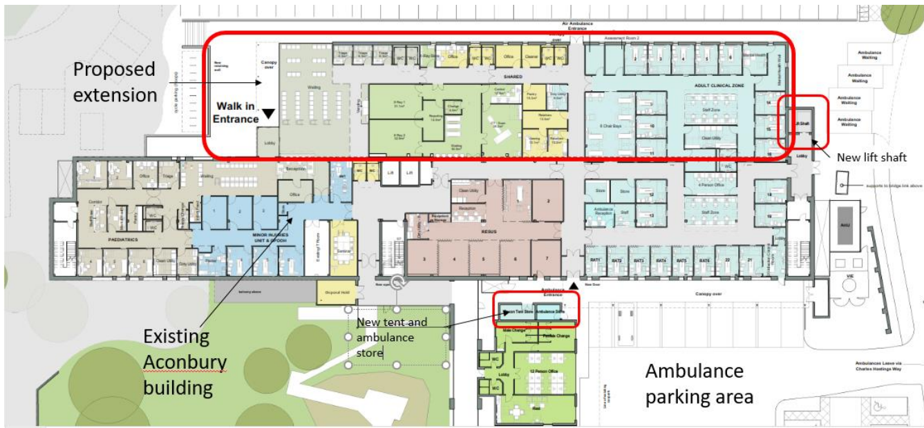
Figure 2. Proposed ground floor plan with proposed new extension shown in large red box and other smaller development shown also in red areas.
